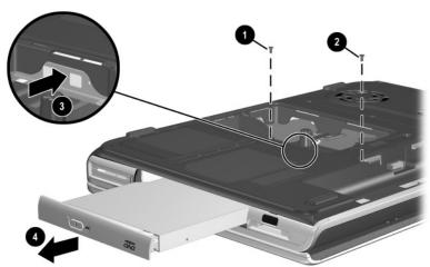
Removing the Optical Drive
